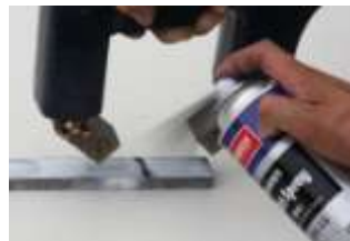
4. Spray SM-15 (black Magnetic particle)
