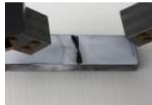
5. Examine the defective area with naked eye
