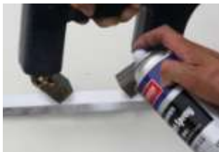
3. Forming the magnetizing current magnetic field
