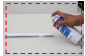
2. Spray MP-35 (White Paint)
