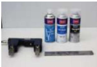
Testing Equipment & Magnetic particle Detecting Spray
